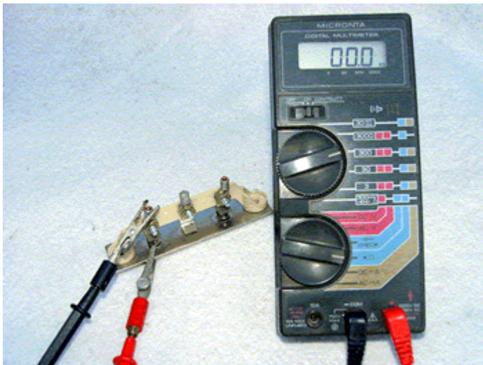
Image 3 - Second step of checking diode.
